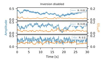
Fig. 16. Time series of a single OFDM subcarrier from Wi-Fi measurements and  $1\,\mathrm{s}$  sliding-window standard deviation for various values of R. The inversion step of Algorithm 1 is bypassed.
