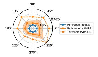
Fig. 13. Effect of IRShield on the adversarial reference measurement for varying IRS orientations. The IRS faces towards the eavesdropper at  $0^{\circ}$ . We plot the median and the  $1^{\text{st}}$  and  $99^{\text{th}}$  percentiles of the adversarial observations and the resulting motion-detection threshold according to [37] with C=11.
