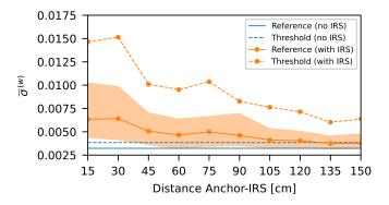
Fig. 12. Effect of varying distances of the IRS to the anchor device. We plot the median and the 1<sup>st</sup> and 99<sup>th</sup> percentiles of the adversarial observations and the resulting motion-detection threshold according to [37] with C=11.
