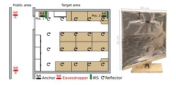
Fig. 21. Measurement setup of the coverage test, indicating the 20 rotating reflector positions (left) and the rotating reflector on a wooden frame (right).
