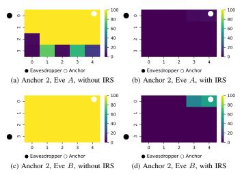
Fig. 9. Spatial distribution of detection rates for anchor position 2 with motion-detection threshold according to [37] with C=11.
