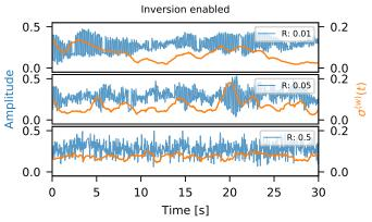
Fig. 17. Time series of a single OFDM subcarrier from Wi-Fi measurements and  $1\,\mathrm{s}$  sliding-window standard deviation for various values of R.
