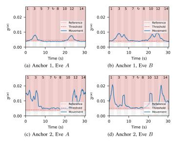
Fig. 4. Adversarial motion sensing results for eavesdropper positions A and B, receiving signals from anchor 1 and 2 with a person walking along a predefined path (see the numbering in Fig. 3). We plot the channel sliding-window standard deviation observed by the adversary with and without movement in the target area.
