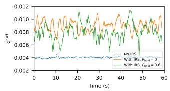
Fig. 6. Illustration of the effect of IRShield on the adversarial channel observation. We plot the channel sliding-window standard deviation with and without IRShield.
