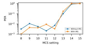
Fig. 14. Packet error rates over MCS setting without and with IRShield when a legitimate party receives packets from an anchor device. A higher MCS value indicates a higher data rate transmission.
