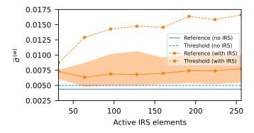
Fig. 11. Effect of varying number of active IRS elements. We plot the median and the  $1^{\rm st}$  and  $99^{\rm th}$  percentiles of the adversarial observations and the resulting motion-detection threshold according to [37] with C=11.
