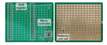
Fig. 5. Intelligent reflecting surface prototype  $(43 \times 35 \text{ cm})$ . Back side with control circuitry (left) and front side with reflecting elements (right).
