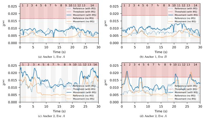
Fig. 7. Adversarial motion sensing results with IRShield active. We plot the channel sliding-window standard deviation observed by the eavesdropper during the reference measurement without motion and with a person walking along a pre-defined path (see the numbering in Fig. 3). Also, we indicate the motion-detection threshold according to [37] with C = 11. For comparison, we also plot the results when IRShield is not active, cf. Fig. 4.
