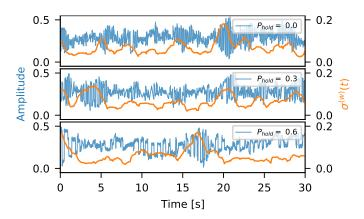
Fig. 18. Time series of a single OFDM subcarrier from Wi-Fi measurements and  $1\,\mathrm{s}$  sliding-window standard deviation for various values of  $P_{\mathrm{hold}}$ .
