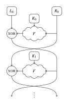
Figure 5: DFG of a Feistel structure
