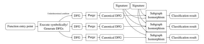
Figure 2: Diagram of primitive identification process
