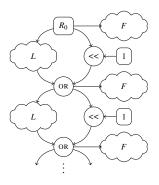
Figure 6: DFG of an (N)LFSR
